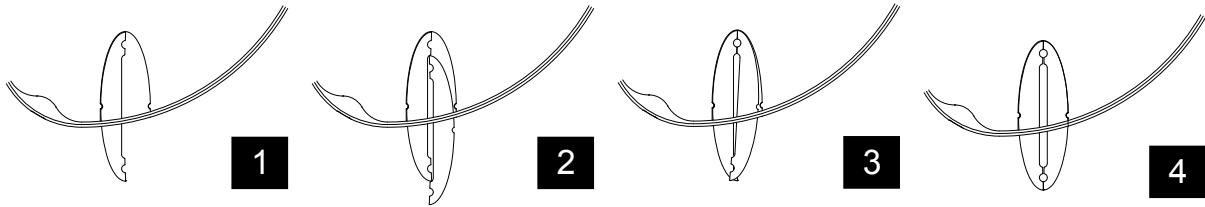
To insert the blades, first insert one blade, then the other. To fully seat the second blade, cross it over the first one, as shown in the drawings above. A small amount of force may be required, but do not use tools, as that might impart an excessive amount of force. Finally, slide the plastic clip over the blades, insert the screw and tighten the wingnut.
